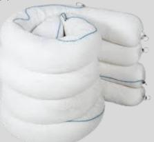
Bullman oil absorbent net boom are made an outer plastic netting that contains a spun bond inner sock which filled with recycled polypropylene. It can be used either on land or water to block the spillages. Oil absorbent boom is used to absorb and contain oil. A strong mesh outer sleeve encases a poly sock skin filled with highly sorbent poly blend. Booms won't shed or sink, even when saturated with oil.
