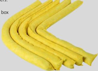
Bullman Chemical absorbent sock ideal for use as a barrier to encircle a spill or placed around the base of drums and machinery to absorb any nuisance leaks or drips. Suitable for absorbing aggressive fluids including acids and alkalis. Spunbond outer sleeve is both fast wicking and tough. The absorbent core is secured into the sock at each end with a stitched seam.
